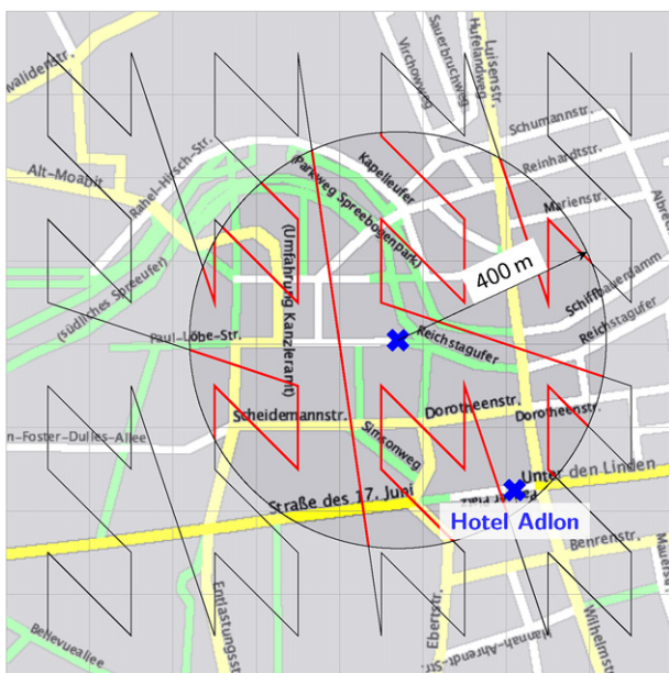
Fig. 4. 2-Dimensional range query using z -curves.
