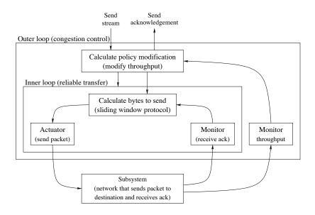
FIGURE 2: TCP as a feedback loop structure
